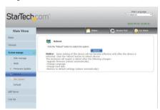
3. The Reboot window is now displayed. From the reboot Window you can remotely reboot the system through the web interface.
